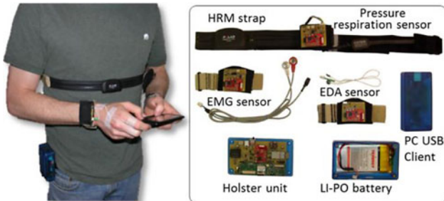
Fig. 2. Snapshot of a subject wearing the full sensor suite. The chest strap is shown outside the shirt for illustration purposes. The system consists of a holster unit, a chest strap combining HRM and respiration sensors, and wireless EMG and EDA modules. A USB transducer can be used to display sensor data in real-time on a PC monitor during sensor calibration.
