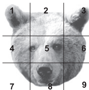
Fig. 4. Nine subregions used for feature extraction, which roughly correspond to different parts of animal faces such as ears, eyes, and cheeks.
